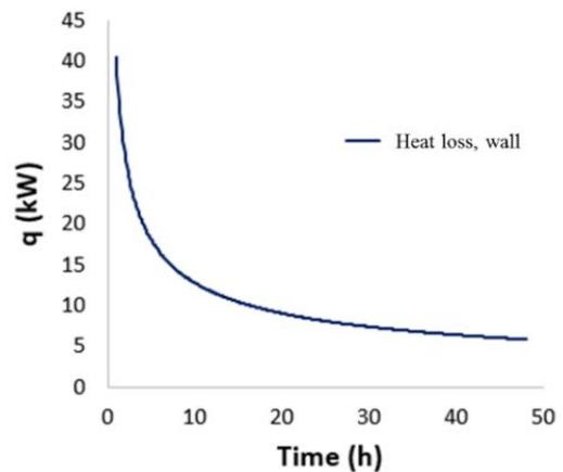
Fig. 2 Rate of conductive heat loss through the wall
