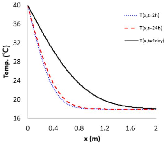
Fig. 3 Temperature distributions on the concrete wall
