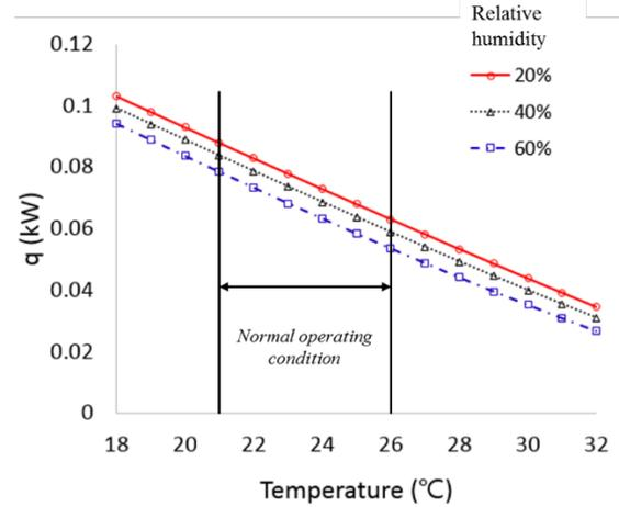
Fig. 4 Rate of heat losses by evaporation
