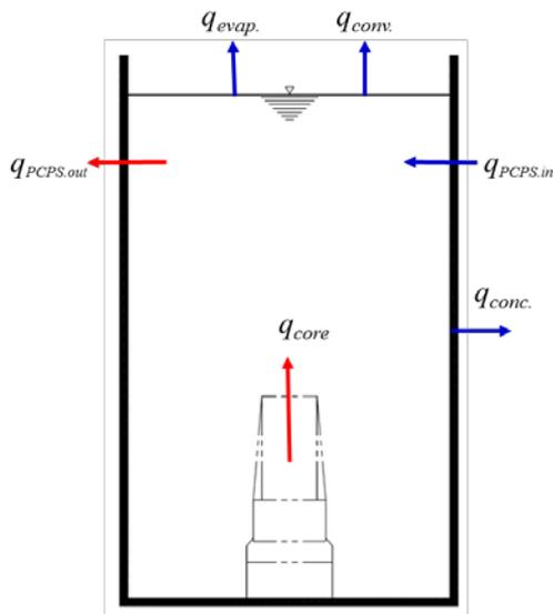
Fig. 1 Schematic of an open pool type reactor
