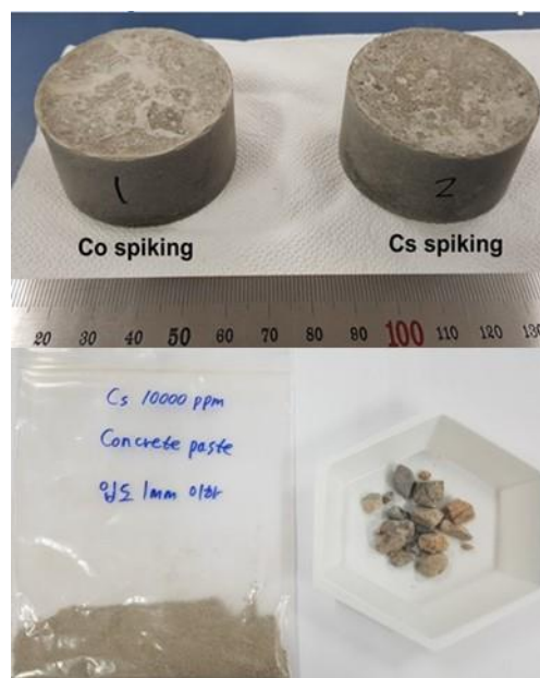
Fig. 1. Prepared concrete sample spiked by Co or Cs (Top) and separation of concrete pastes from aggregates (Bottom)
