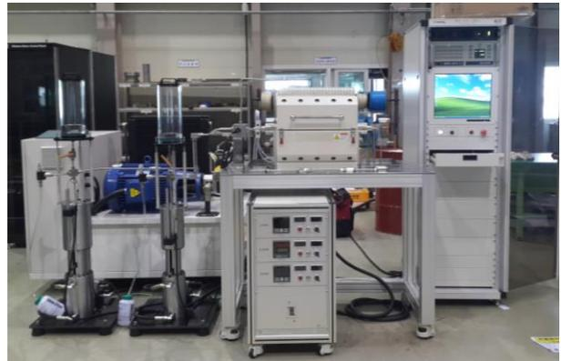
Fig. 1. Photograph of the fatigue tester under internal pressurization on the cladding tube.
