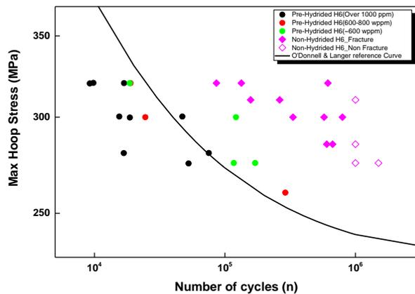
Fig. 2. Fatigue curve (Stress-Number of cycle curve) of the pre-hydrided/non-hydrided HANA-6 cladding tube.
