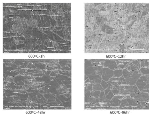
Fig. 4. Microstructure observation after EPR test.
