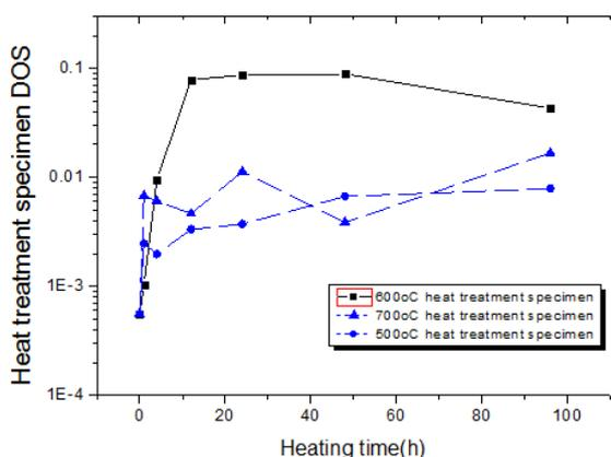
Fig. 3. Ratio of reactivation current density to activation current density ( $I_r/I_a$ ) as a function of heat treatment time
