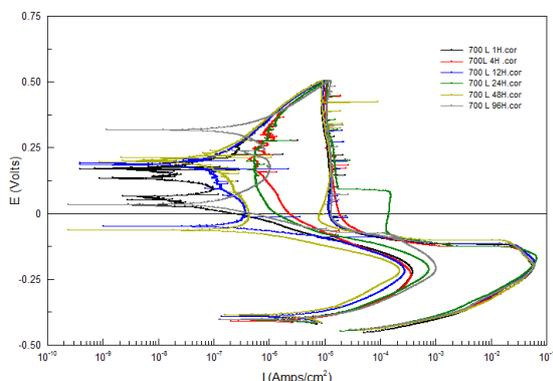
Fig. 2. Double loop EPR curves for specimens heat treated at 700°C.
