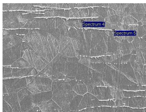
Fig. 1. Microstructure at plane perpendicular to rolling direction of the as received specimen etched oxalic acid.
