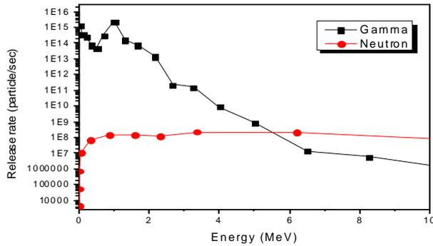
Fig. 1. Gamma and Neutron release rate of 12 assemblies
