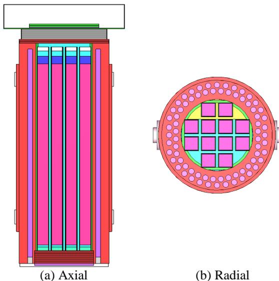
Fig. 2. KN-12 cask modeled with SCALE 6.1
