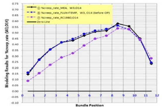
Fig. 5. Comparison of pressure tube diameter prediction results
