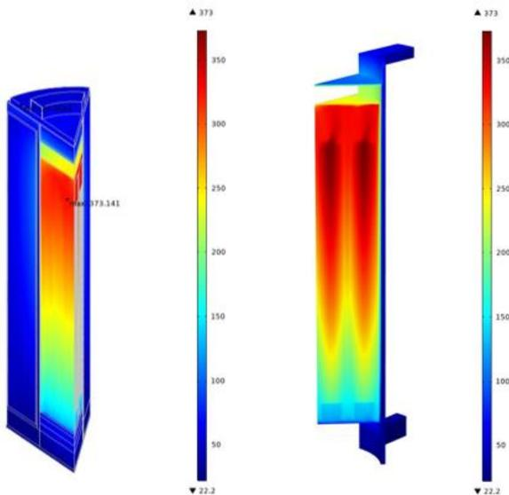
Fig.7. 3D temperature profile of HISTORM-100 cask with WH14X14 heterogeneous fuel assemblies
