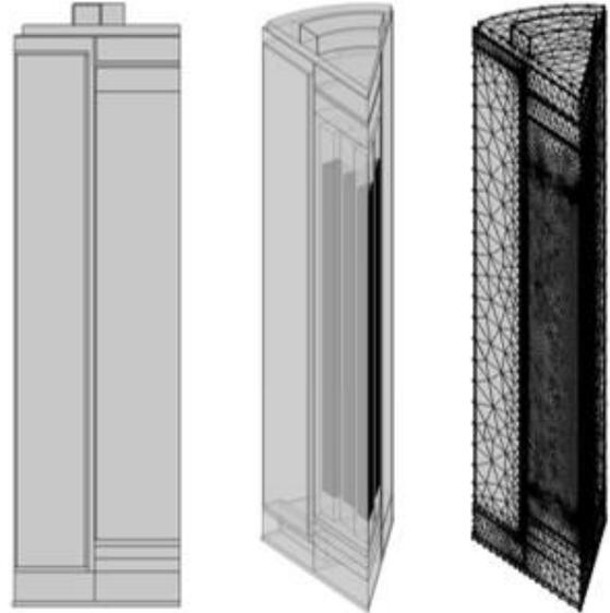
Fig.1. Geometry and mesh of HISTORM-100 cask with WH14X14 heterogeneous fuel assembly
