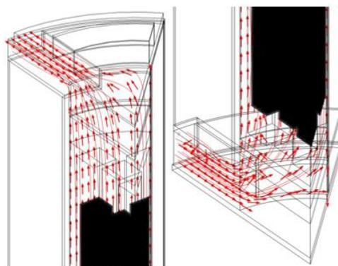
Fig.5. Air flow distribution inside the cask
