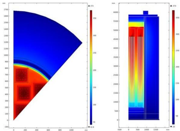
Fig.6. 2D temperature profile of PCT height cutting plane and 2D temperature profile of 45° cutting plane
