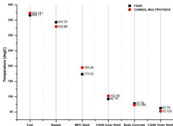
Fig.2. Comparison of FSAR and COMSOL MULTIPHYSICS results
