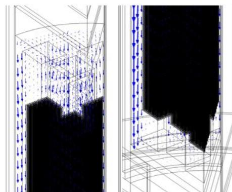
Fig.4. Helium flow distribution inside the canister
