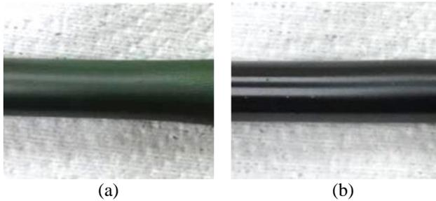
Fig. 2. Photographs of Zr cladding specimens (a) with and (b) without Cr coating after high temperature oxidation.
