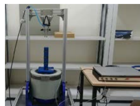
Fig. 1. Vibration packing system with the feeding apparatus of the metal powder.
