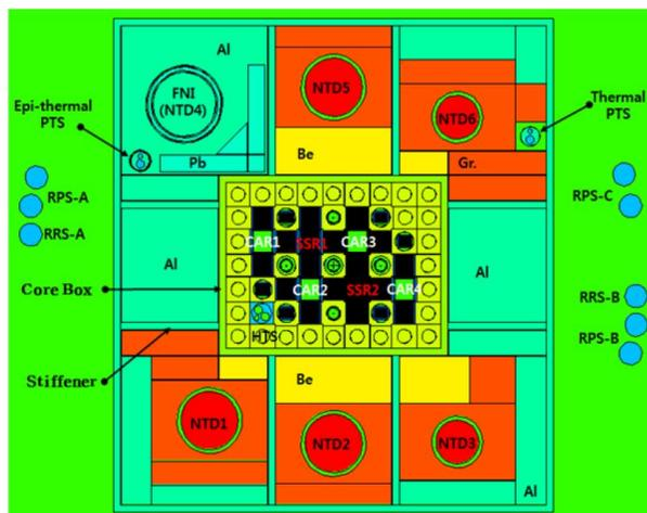
**Figure 1.** KJRR Core Configuration
