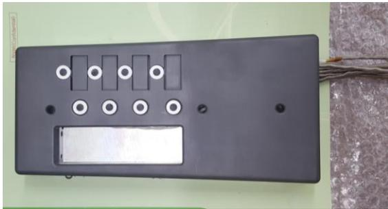
Figure 7. Photo of the Langmuir probe array.
