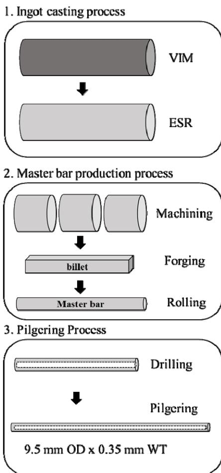
Fig. 3. Thin tube manufacturing process for ADSS and AFS.
