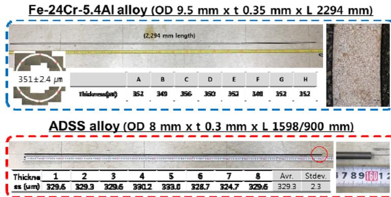
Fig. 2. Photo of FeCrAl tube fabricated by pilgering with a dimension of 9.5 mm OD x 0.35 mm t x 1.9 m L.
