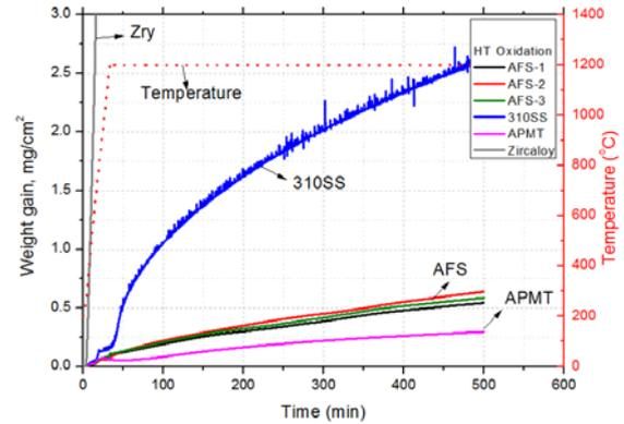
Fig. 1. Oxidation test results of AFS alloys tested in 1200 °C Ar/steam mixed environment.
