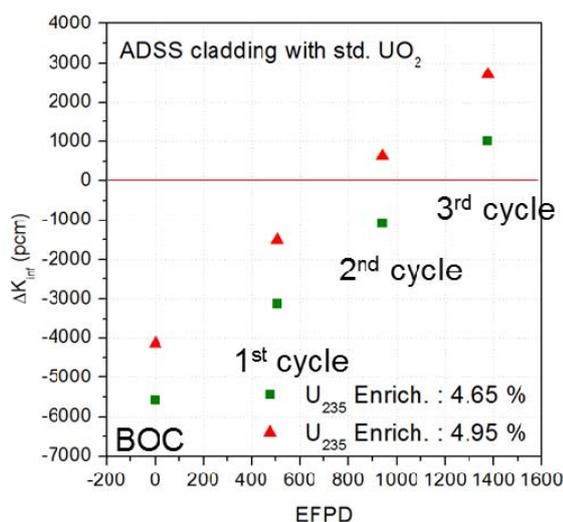
Fig. 4. The difference of multiplication factor of ADSS cladding with 0.35 mm thickness compared to current  $\text{UO}_2/\text{Zr}$  fuel system.
