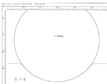
Fig. 5 Groove measurement result (Test No.1)
