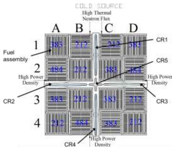
Fig. 1. Core arrangement of OPAL reactor
