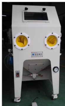
Fig.1. Sandblasting equipment and operation conditions.
