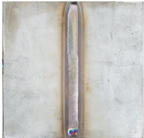
Fig. 2. Photographs of the welded specimen and magnified images on the surface of with and without HFNP treatment
