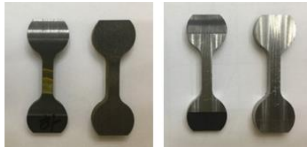
Fig. 3. Fabricated transverse tensile testing specimens from an unirradiated pressure tube prior to CNC Mill (left) and after removal of a heat affected zone (right).
