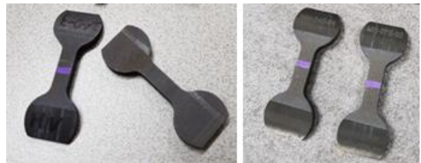
Fig. 4. Transverse tensile testing specimens with the identification number labelled by an ink felt marker (left) and by the ID laser engraved system (right).
