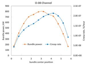
Fig. 2 Typical axial distribution of PT creep rates and bundle power
