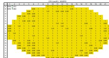
Fig. 8 CPR ratio (Lee data/RC1980 data) map for 3650 FPD of W-4
