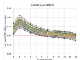
Fig. 4 PT creep ratio (Lee model/RC1980) above 6.0 MW of channel power at 3650 FPD
