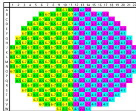
Fig. 1 Core fuel channel distribution
