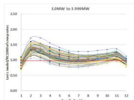
Fig. 3 PT creep ratio (Lee model/RC1980) between 3.0 MW and 3.99 MW of channel power at 3650 FPD
