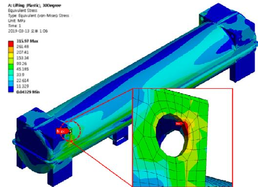
Fig. 4. Equivalent stress for lifting analysis result
