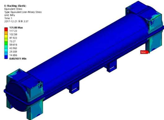
Fig. 3. Equivalent stress for stacking analysis result
