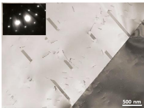
Fig. 2. TEM image showing a dislocation morphology in the non-irradiated 316 SS.
