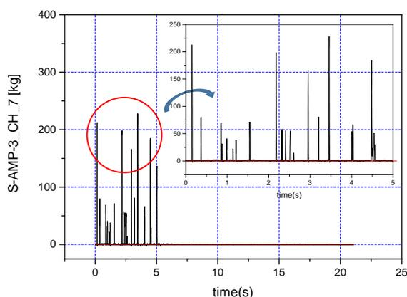
Figure 4. Impact force history of fuel storage rack "H" under SSE, 60% water level condition.
