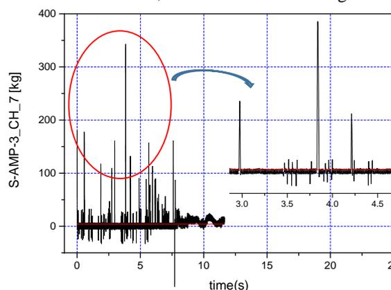
Figure 5. Impact force history of fuel storage rack "H" under BDBE, 60% water level condition.
