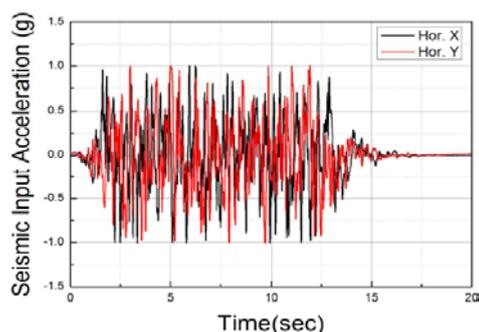
Figure 2. Standard seismic input acceleration time history.
