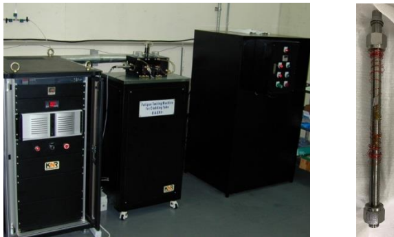
Fig. 1. Device for applying pressure and tube specimen.
