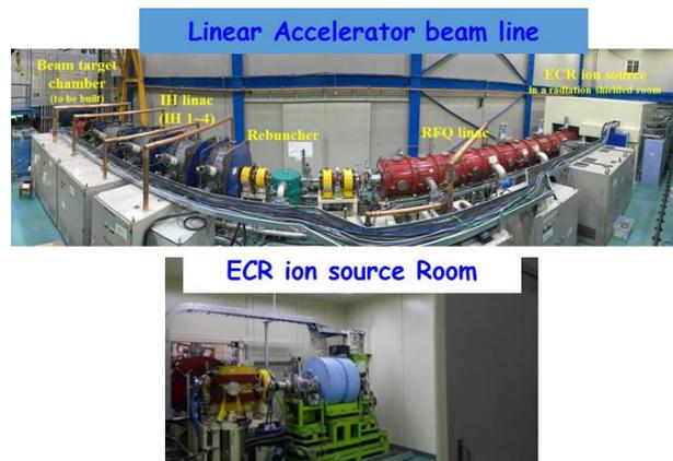
Fig. 2. The assembled linear accelerator system
