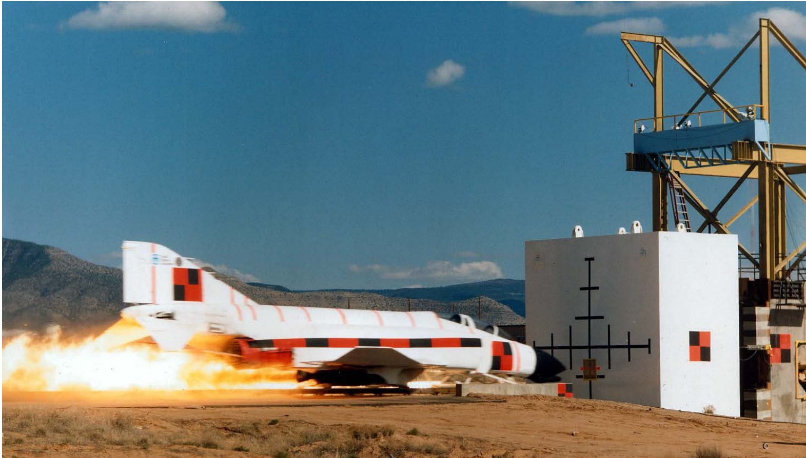
Figure 2: Impact of a fighter plane on a concrete wall, © Sandia National Laboratories
