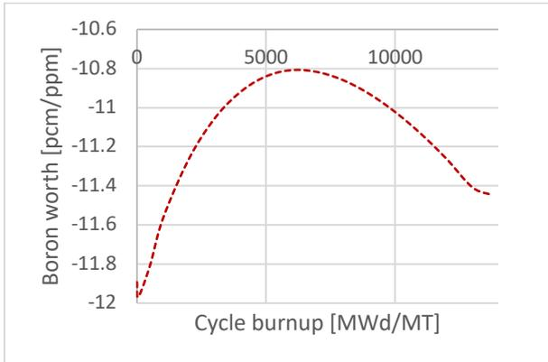
Fig. 6. Boron worth vs. cycle burnup
