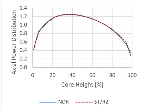
Fig. 2. Average axial power distribution at BOC
