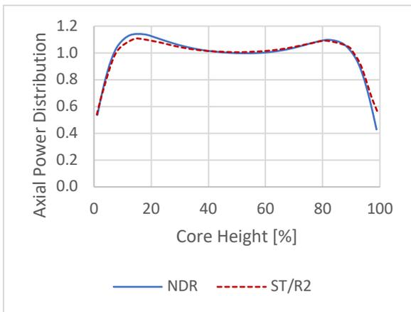
Fig. 3. Average axial power distribution at EOC
