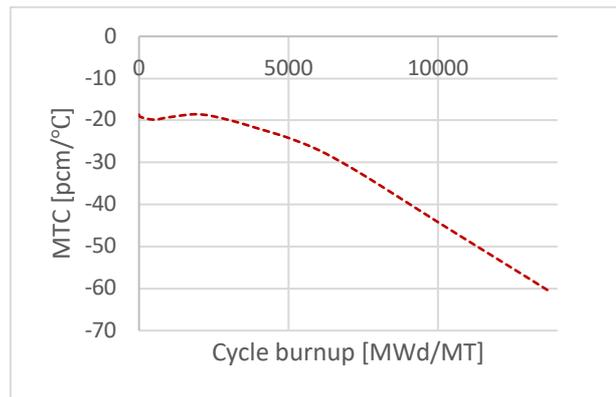
Fig. 8. MTC vs. cycle burnup
