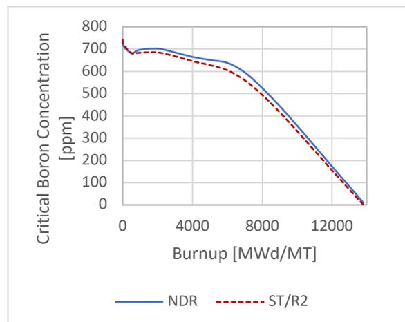
Fig. 1. Critical boron concentration vs. cycle burnup
