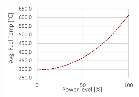
Fig. 7. Average fuel temperature as a function of power
