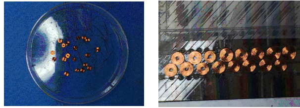
Fig. 5. ECA probe coil winding and arrangement
