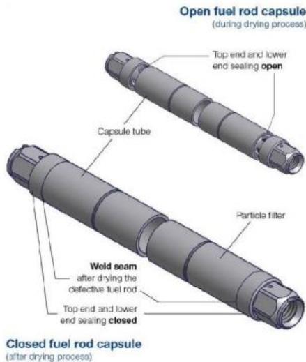
Fig. 3. Framatome (AREVA NP) opened and closed fuel rod capsules
