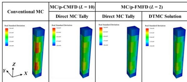
Figure 4 Comparisons of real SDs in one-group fine-mesh flux distributions for three test cases.
