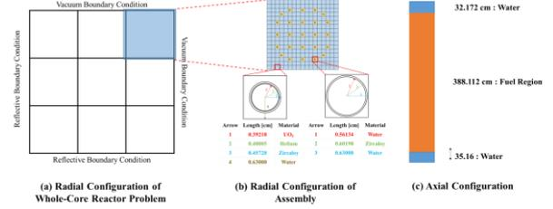
Figure 2 Configurations of continuous-energy three-dimensional reactor test problem.
