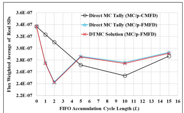
Figure 3 Flux weighted average of real SDs in one-group integrated fine-mesh flux distributions, where the FIFO accumulation cycle length  $L = 0$  indicates the results from the conventional MC.
