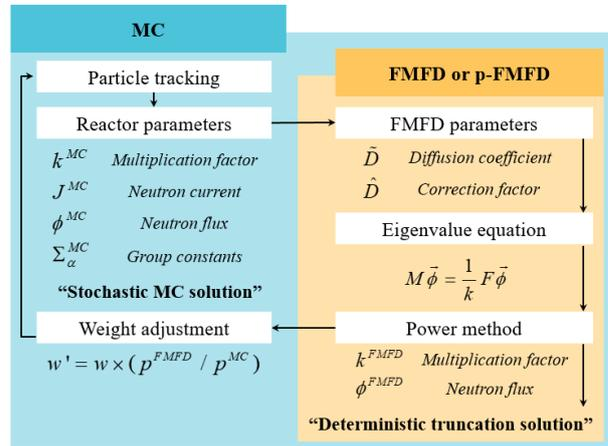
Figure 1 Flow chart of MC/FMFD (or p-FMFD) and DTMC method.
