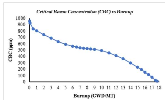
Fig. 3. Boron Concentration as a function of burnup.
