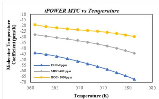
Fig. 4. Moderator Temperature Coefficient in iPOWER.
