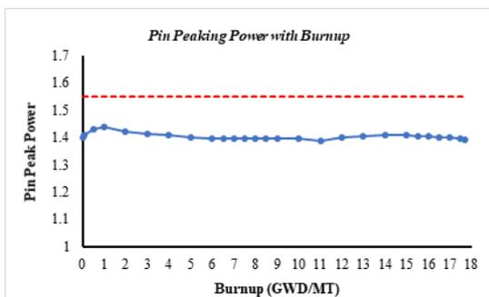
Fig. 2. Maximum rod relative power to core average rod power as a function of burnup.
