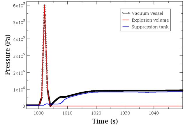
Fig. 1. Pressure transient results of single explosion accident with LOCA accident
