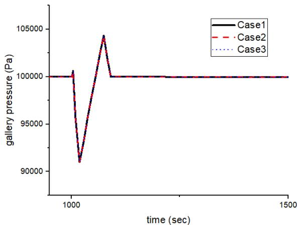
Fig. 3. Pressure transient inside gallery for each Case.
