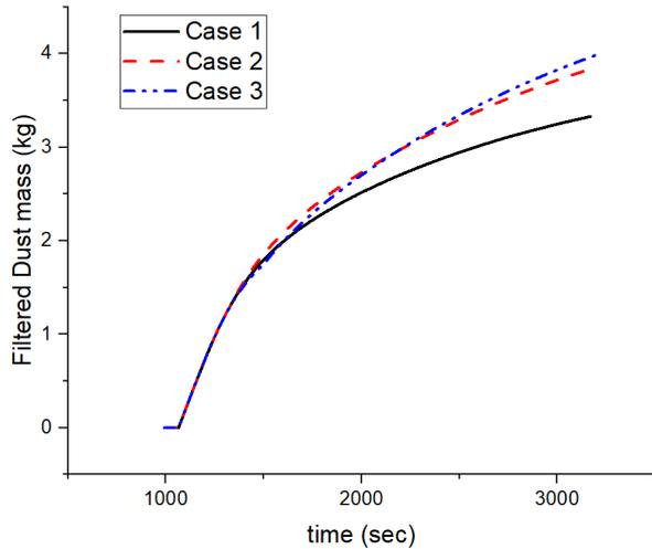
Fig. 2. Filtered dust mass through detritiation system between environment and gallery volume.
