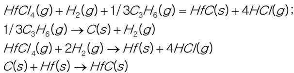
Fig. 1 shows the equilibrium phases depending on the temperature at 1200°C, 6.7 kPa. HfC begins to form at about 500°C and HfCl<sub>4</sub>:C<sub>3</sub>H<sub>6</sub>:H<sub>2</sub> = 3:0.32:100. A near-single phase HfC forms above 1200°C, as shown in Fig. 1(a). Fig. 1(b) shows the C/HfC ratio in HfC-1 and HfC-2 deposition conditions. The amount of excess carbon decreases as H<sub>2</sub> increases.
