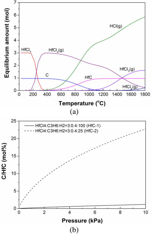
Fig. 1. (a) Equilibrium phases and (b) C/HfC ratio in the HfCl<sub>4</sub>-C<sub>3</sub>H<sub>6</sub>-H<sub>2</sub> system [4].
