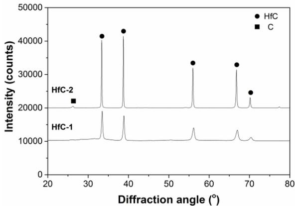
Fig. 2. X-ray diffraction peaks of hafnium carbides.
