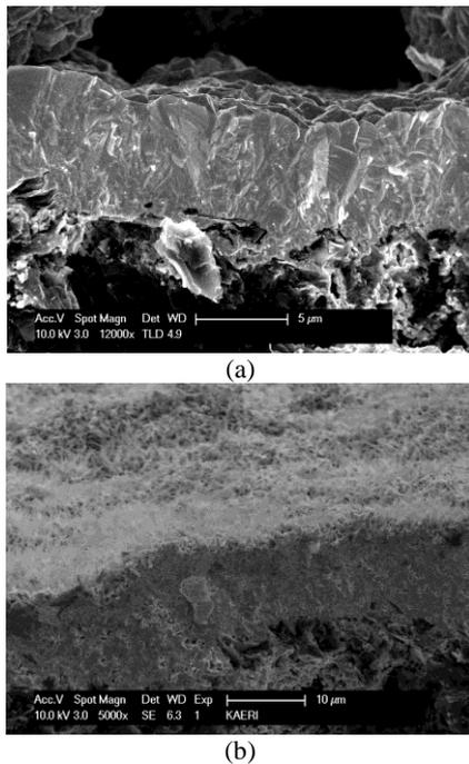
Fig. 3. Microstructures of HfC coatings: (a) HfC-1 and (b) HfC-2.
