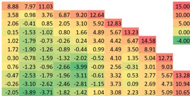
Fig. 7. Power error (%) from the reference and FWC with no DF for 2-D benchmark.
