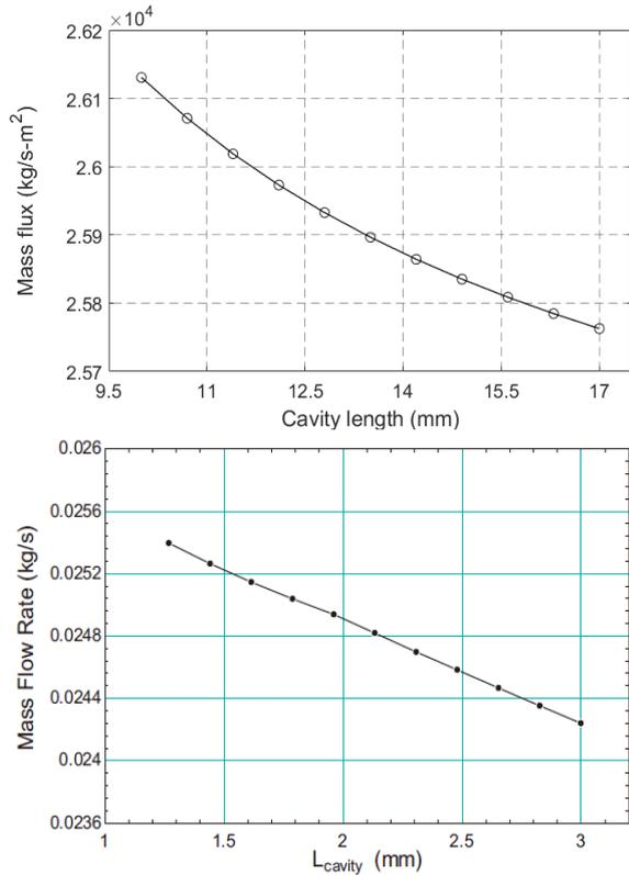
Fig 5. Mass flux change with cavity length (upper: KAIST, bottom: University of Wisconsin-Madison[4])
