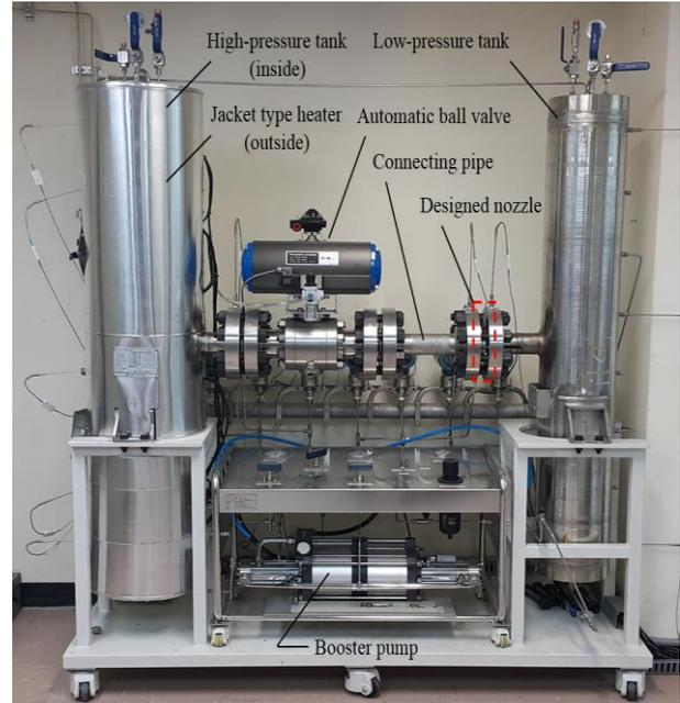
Fig. 1. S-CO<sub>2</sub> critical flow experimental facility
