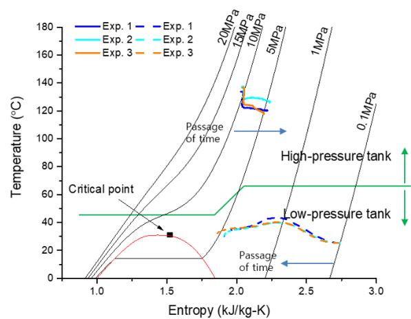
Fig 7. T-s diagram of high- and low-pressure tank
