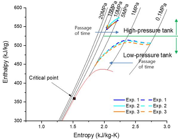
Fig 8. h-s diagram of high- and low-pressure tank
