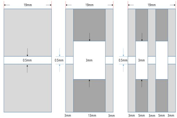
Fig. 2. Internal geometry of labyrinth seal geometry nozzle
