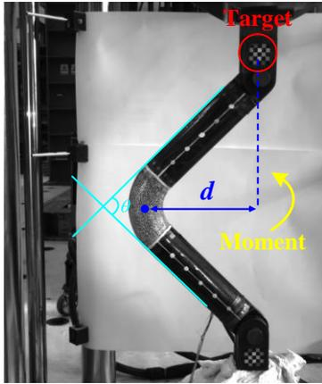
Fig. 3 Theta measurement using MATLAB
