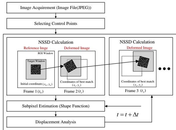
Fig. 1 Displacement measurement algorithm
