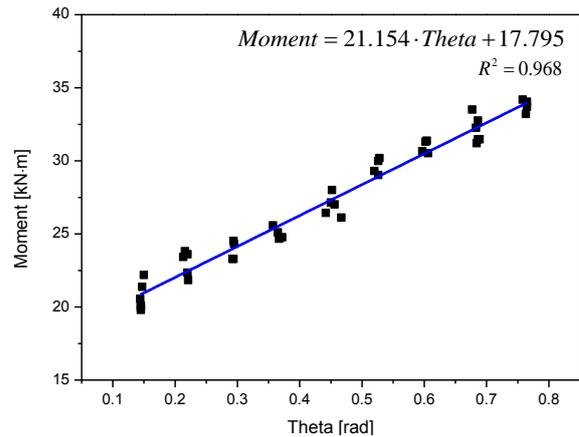
Fig. 5 Leakage line using moment-theta
