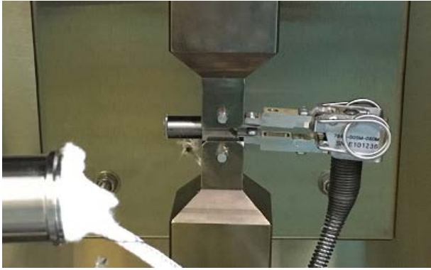
Fig. 3. COD gage mounted on PLT fixtures
