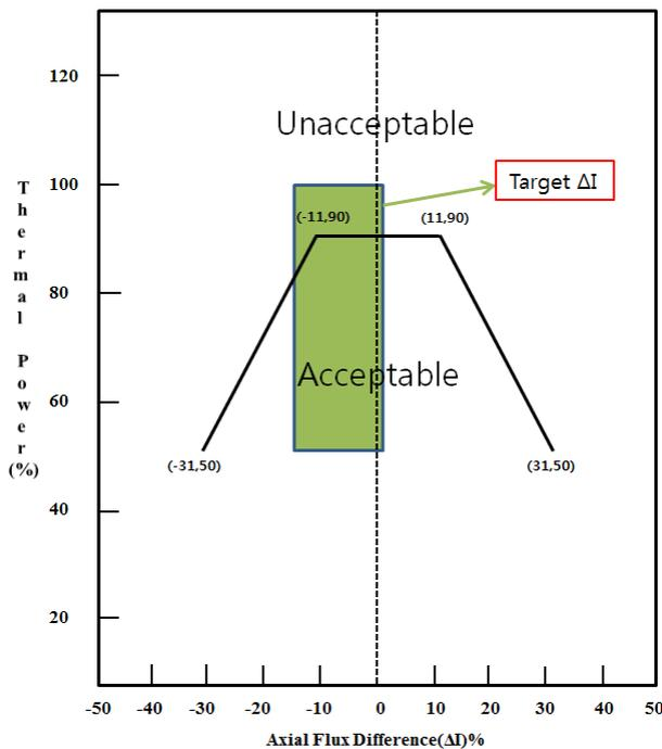
Figure 1 Technical Specification Limits of AFD
