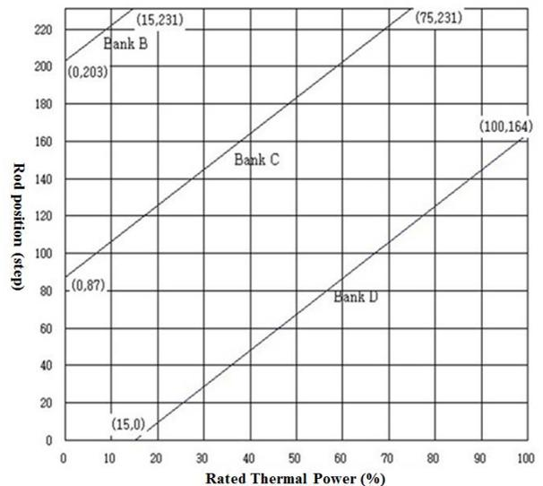
Figure 2 Power dependent rod insertion limit
