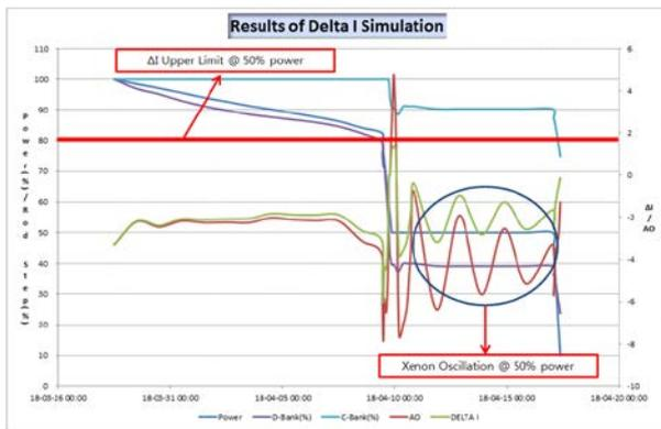
Figure 3 Results of Delta I Simulation
