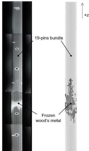
Fig. 4. Experimental and numerical simulation result for frozen Wood's metal distribution in 19-pins bundle.
