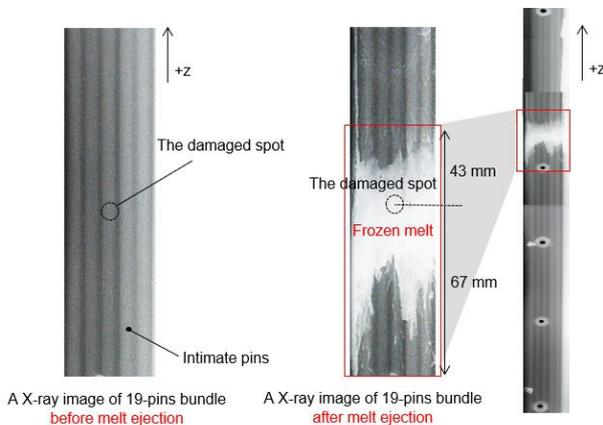
Fig. 2. Radiographic images of frozen Wood's metal before and after melt ejection.
