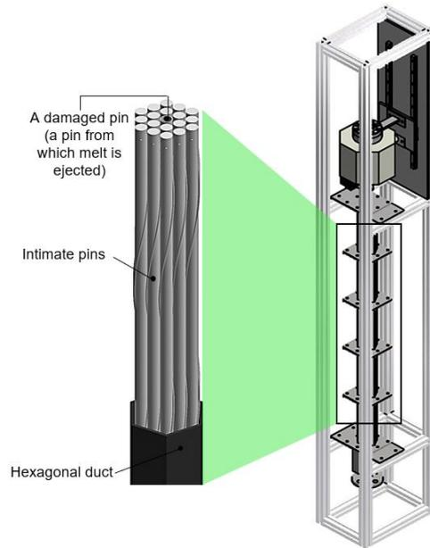
Fig. 1. Schematic diagram of UNICORN.
