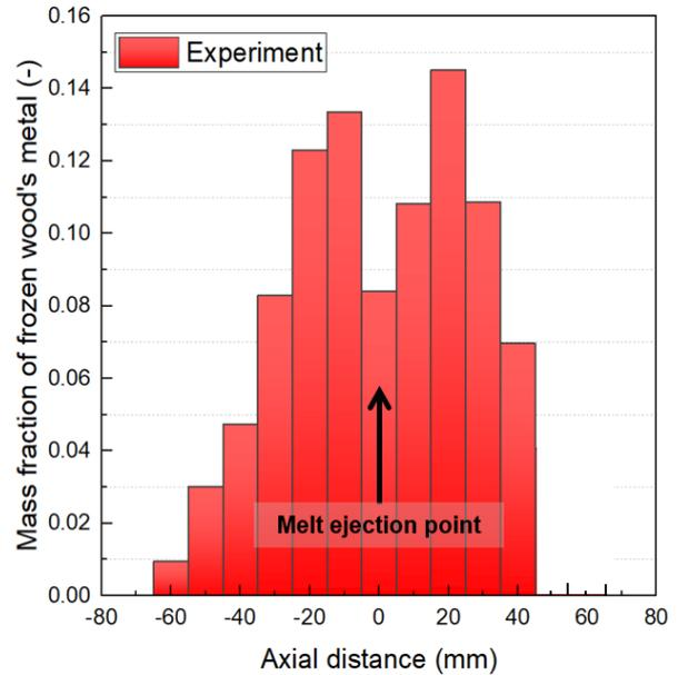
Fig. 3. Mass fraction of frozen Wood's metal along axial distance.
