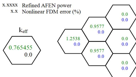
Fig. 4. Results of the mini core problem (1/6 core)
