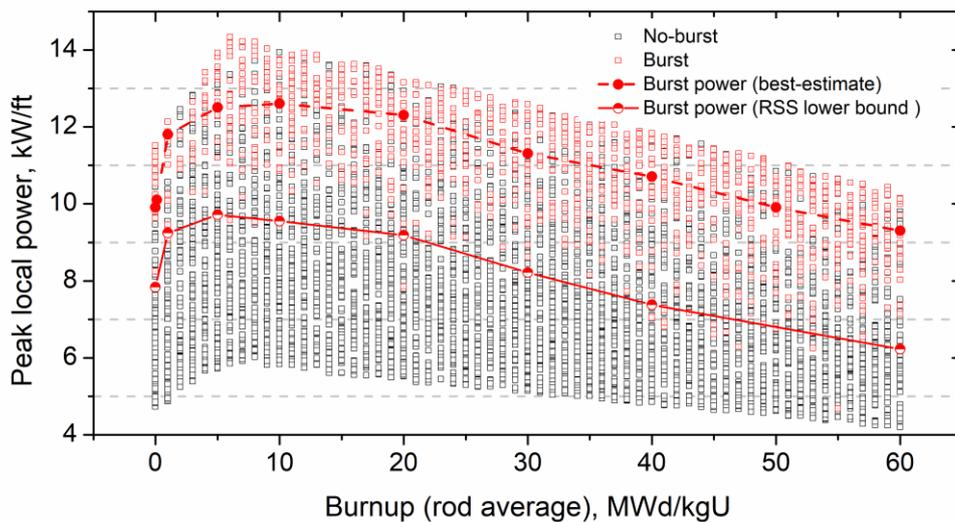
Fig. 2. Preliminary assessment of rod burst power with combined uncertainty and lower bound of power curve within licensing fuel burnup of 60 MWd/kgU.
