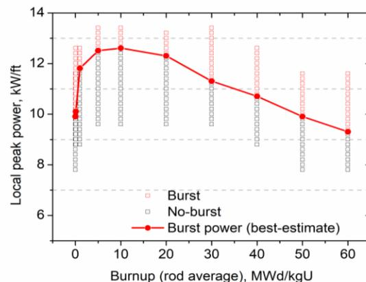
Fig. 1. Best-estimate required peak fuel power for rod burst as a function of fuel burnup.
