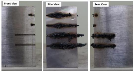
Fig. 2. Underwater laser cutting of 60-mm-thick stainless steel. Stand-off distances are 10mm, 10mm, 5mm, 2mm from top to the bottom. Focal point position correspond to 0mm, 0mm, -5mm, -8mm from top to the bottom
