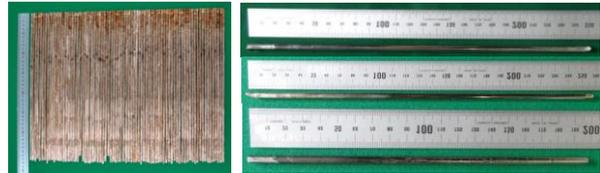
Fig. 2. Cu slugs from engineering-scale injection casting equipment and DU slug from small-scale injection casting equipment
