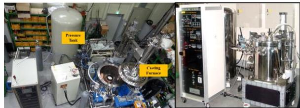
Fig. 1. Engineering-scale injection casting equipment (left) and small scale injection casting equipment (right)
