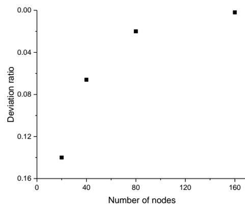
Fig. 1 Node sensitivity in terms of the deviation between FDM and LMTD method
