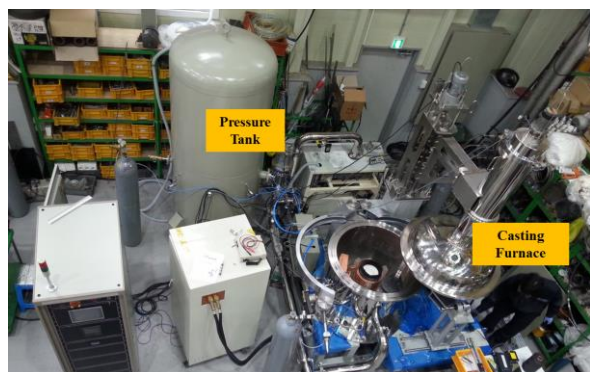
Fig. 1. Engineering-scale injection casting equipment (Max. U-Zr charge: 20kg, installed at KAERI)
