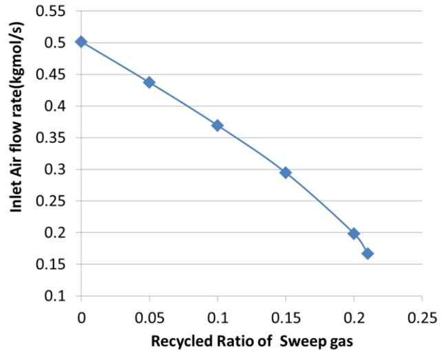
Fig. 4. Inlet Air flow rate as a function of recycled ratio for isothermal boundary condition.
