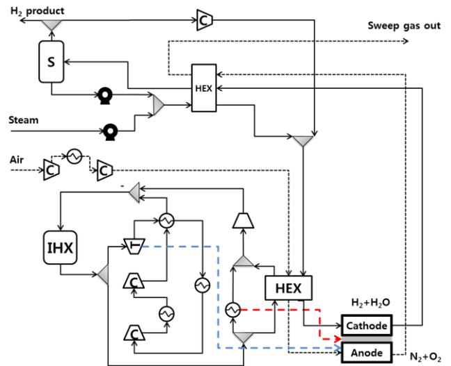
Fig. 1. PFD for HTSE coupled with indirect Brayton cycle
