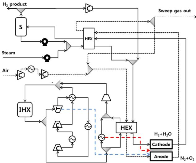
Fig. 2. The proposed PFD including the recycled Anode output stream
