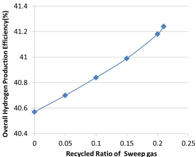
Fig. 3. Overall hydrogen product efficiency as a function of recycled ratio for isothermal boundary condition.
