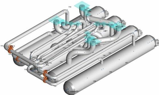
Fig. 1. LP FWH Arrangement in the Condenser Neck
