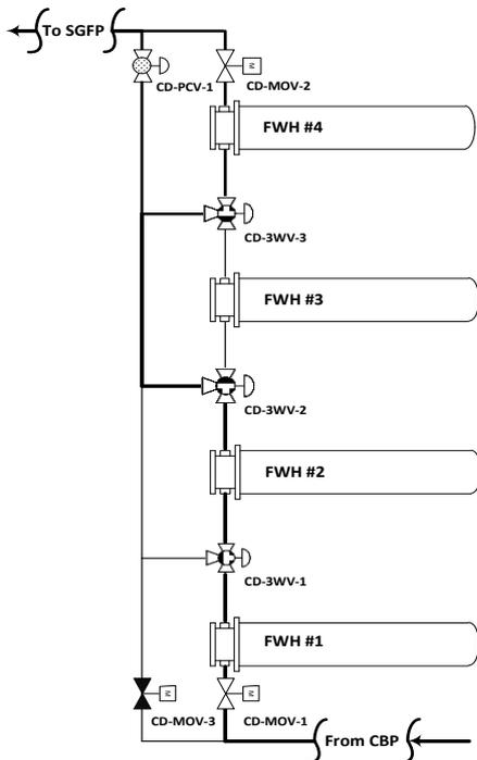
Fig. 2. AM600 LP FWH Bypass Arrangement
