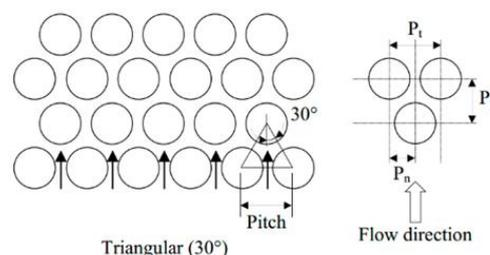
Fig. 3. Tubesheet Standard Pattern
