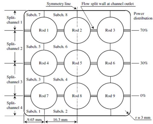
Figure 1. Cross section view of test bundle (Reprinted in Figure 1 of reference 3)
