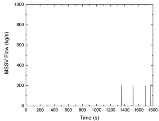
Fig. 5. MSSV flow rate
