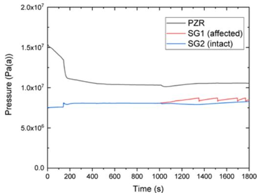
Fig. 3. Primary and secondary pressures
