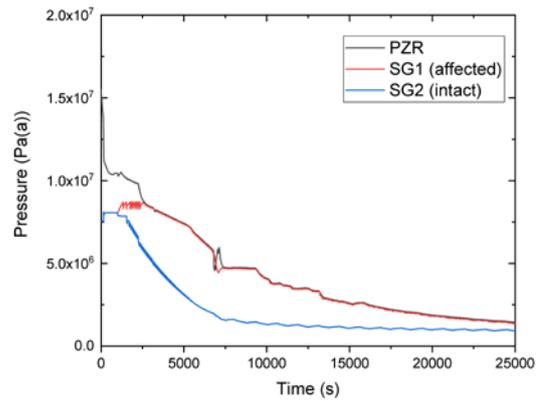
Fig. 8. Primary and secondary pressures
