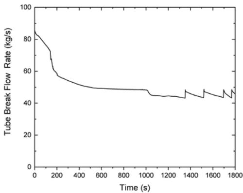
Fig. 2. SG tube break flow rate
