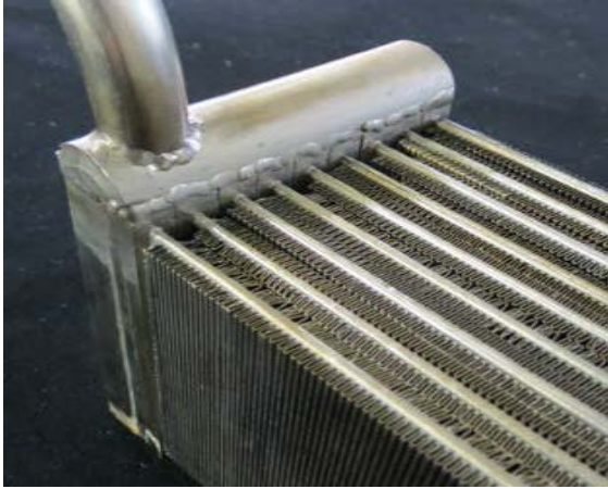
Fig. 5. Many unit cells are connected to manifold [10]
