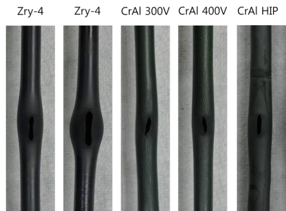
Fig. 1. Appearance of the candidate ATF claddings with various coating layer after integral LOCA test.
