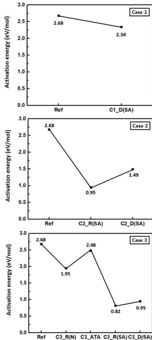
Figure 3. Results of thermal decomposing activation energy of fluoroelastomers in normal operation and SA environment
