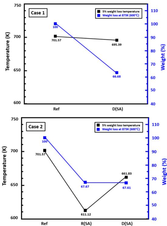
Figure 2. Results of thermogravimetric analysis of fluoroelastomer in normal operation and SA environment (5% weight loss temperature and weight loss at 873K)
